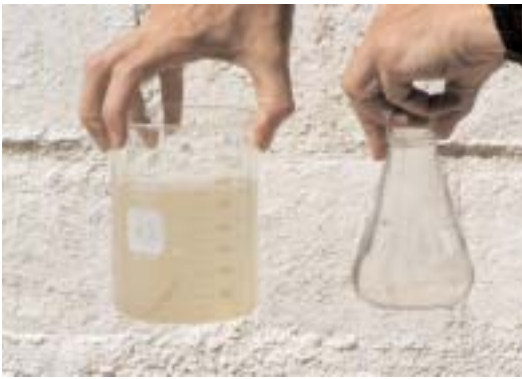
Influent waste water (left) coming into the plant and treated effluent leaving the plant. An air-control system is utilized and odors are generally non-detectable at the plant's property boundaries.
